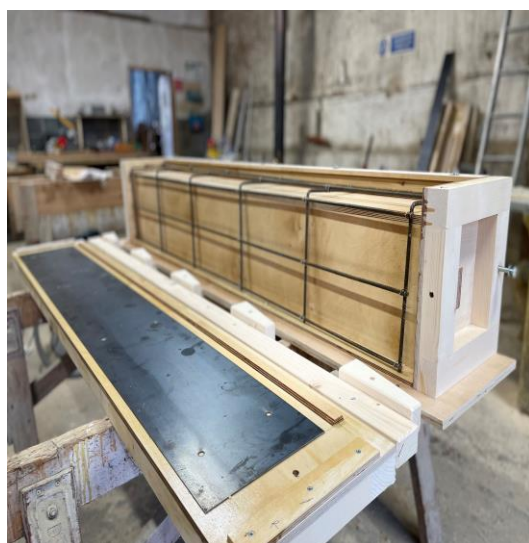
Bespoke Steps and Risers Mould
